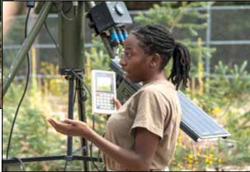
RIGHT: An Airman from the 25th Operational Weather Squadron puts together a TMQ-53 Tactical Meteorological Observing System during seasonal training at Mount Lemmon, Ariz., Sept. 17. The 355th Operations Support Squadron Weather Flight and the 25th Operational Weather Squadron conducted hands-on training with the TMQ-53 to prepare for austere environments to keep the mission going in a deployed location.
