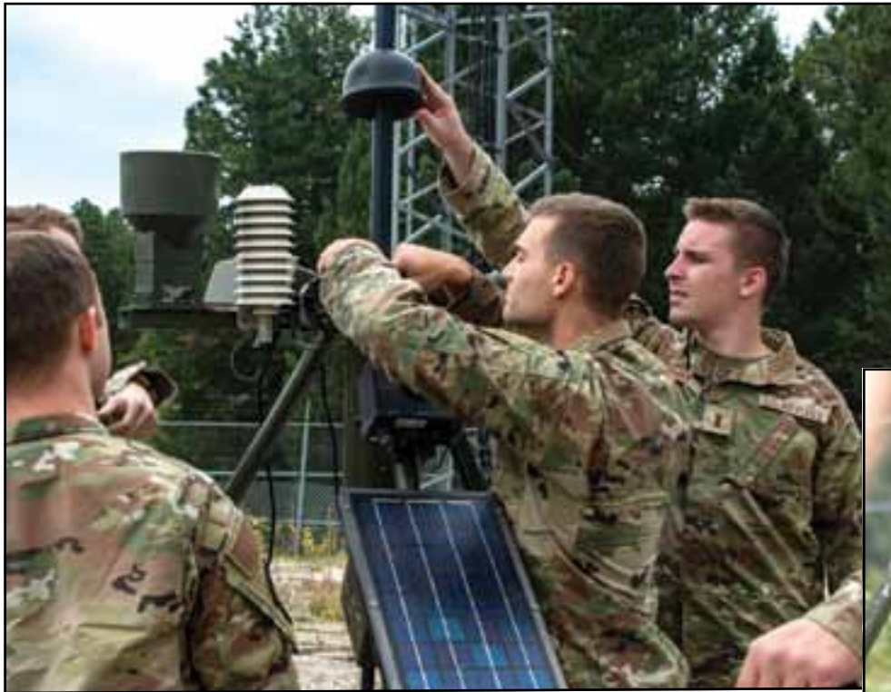
RIGHT: An Airman from the 25th Operational Weather Squadron puts together a TMQ-53 Tactical Meteorological Observing System during seasonal training at Mount Lemmon, Ariz., Sept. 17. The 355th Operations Support Squadron Weather Flight and the 25th Operational Weather Squadron conducted hands-on training with the TMQ-53 to prepare for austere environments to keep the mission going in a deployed location.
